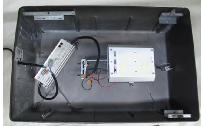
AFTER (shoebox fixture) LED module, driver, L Bracket mount
