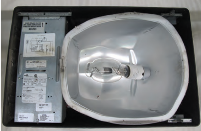
BEFORE (shoebox fixture) ballast box and metal halide
