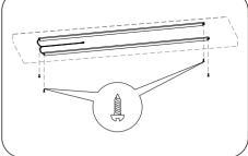
Attach the LED magnetic strip supply directly to the intended mounting surface. Then use the self-tapping screws (provided) at both ends to secure each magnetic strip (optional).
