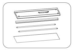
Cut off the power of the troffer retrofit kit before any operation Pull the movable bolt at the edge of the troffer retrofit kit and open the cover.
