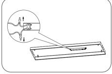
Cut the Line and Neutral wires leading into the existing ballast and leave enough length to make the connection reach the intended location of the LED external driver.
