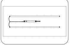
3. Before installing this kit, carefully plan the positioning and lay out of the LED magnetic strip, relative to the expected installation location of the external drive. Route the input wires of the LED magnetic strip to ensure that all input wires can reach the external drive without interfering with the host fixture structural components.
