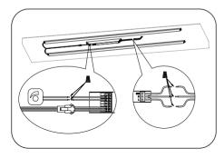
Connect the fixture wires to the supply wires-black to black, white to white, and green to copper/bare.
