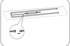
Connect each input lead connector of the LED magnetic strip to the external driver's output lead
