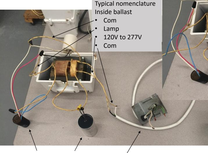
Optional igniter Capacitor Utility power in 120V, 208V, 277V
